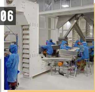
MANUAL SORTING AND METAL DETECTION
